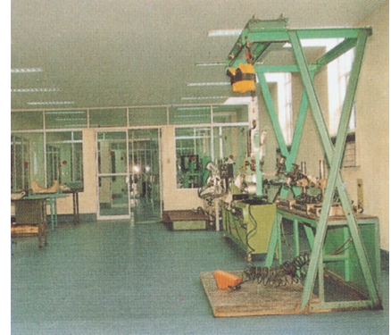
Air-conditioned dust free facility provided for coil making and insulation taping.
